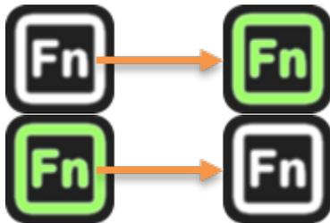
Pressing the **left FN** button activates heating Program 1, turning the button green to indicate it is in use. Pressing the button again during operation will terminate Program 1.
