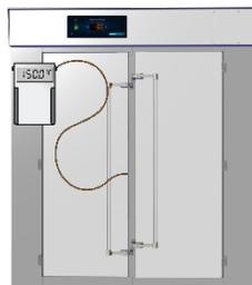
4. The unit must have adequate time to come up to temperature and stabilize. **Failure to wait will result in an inaccurate diagnosis.**
