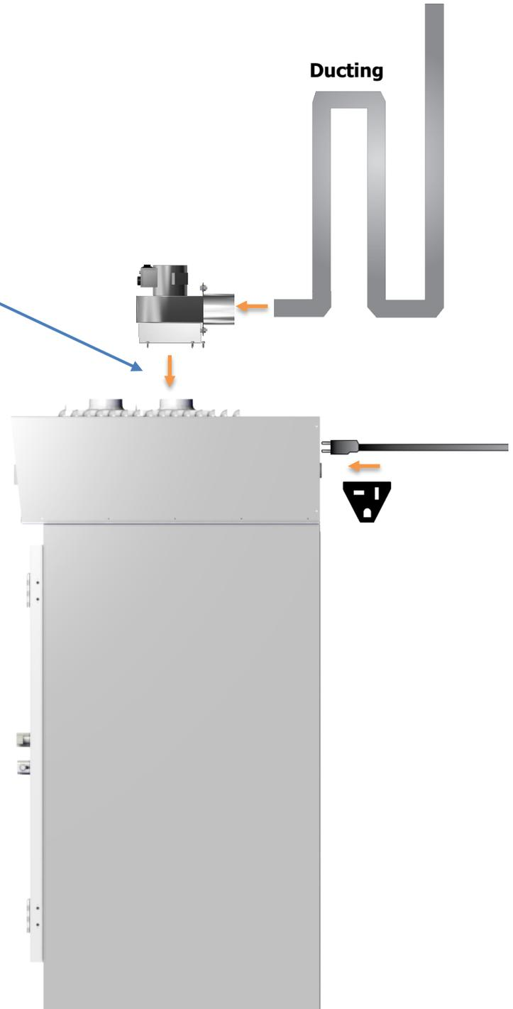
**1.** Remove the 8 screws from the exhaust vent cover on the top, right side of the oven. **Leave the cover in place.**
