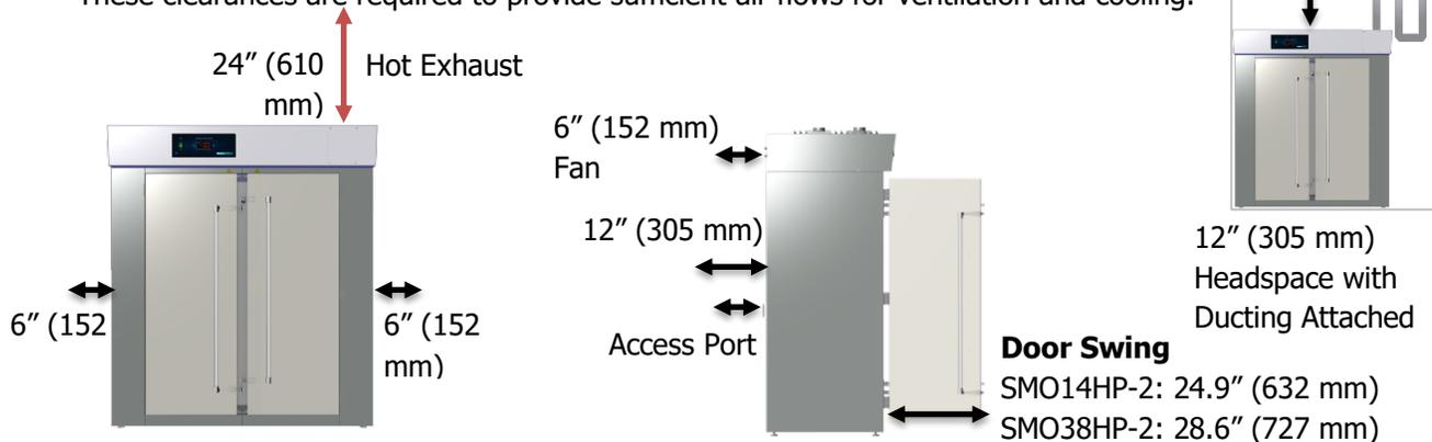
**6 inches (152 mm)** of clearance is required from the sides and the vent fan on the back of the oven. Always ensure the fan is unobstructed.
