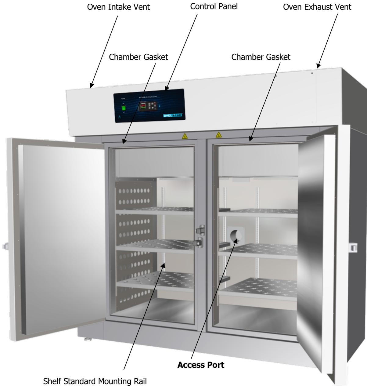
**Note:** The unit has a single oven chamber with two doors.
