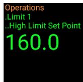
Use the **Set the High Temperature Limit** procedure on page 34 to set the Limit heating cutoff to at least 10°C above the highest intended temperature of your application.
