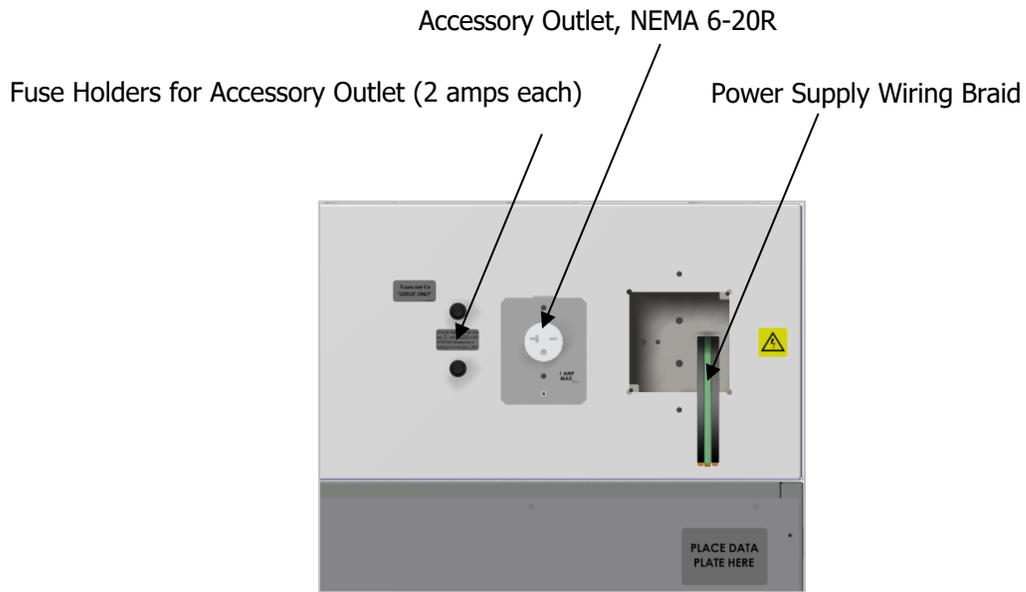
**Permanent Connect Wire Braid 6-gauge, 6 inches (150 mm)**
