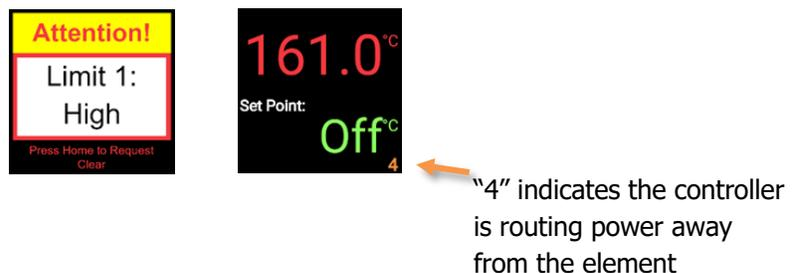
**Alternating alert screens flash when the high limit heating cutoff is active.**
